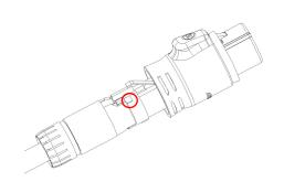
(6) After the assembly of the cable clamp, inner core and housing, tighten the boot in a clockwise direction.
